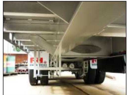
The cross members pass through the main vertical web, as opposed to being stuck on top. This contributes to the strength of the chassis, as the main beams are significantly deeper than other construction methods. The main chassis is then strengthened with a series of cross braces and stiffeners. The end result is an extremely strong platform
